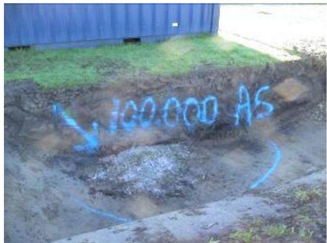
A quick XRF check revealed extreme copper, chromium & arsenic concentrations in some ashes.
